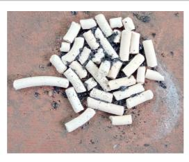
Figure 5. Char deposited HZSM-5 Pellets, 1:0.01, plastic to bentonite ratio
